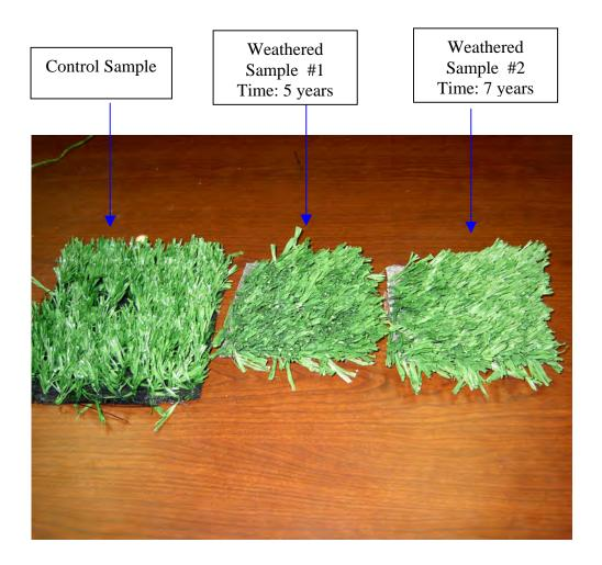
Figure A-1. Control and weathered samples of artificial grass
